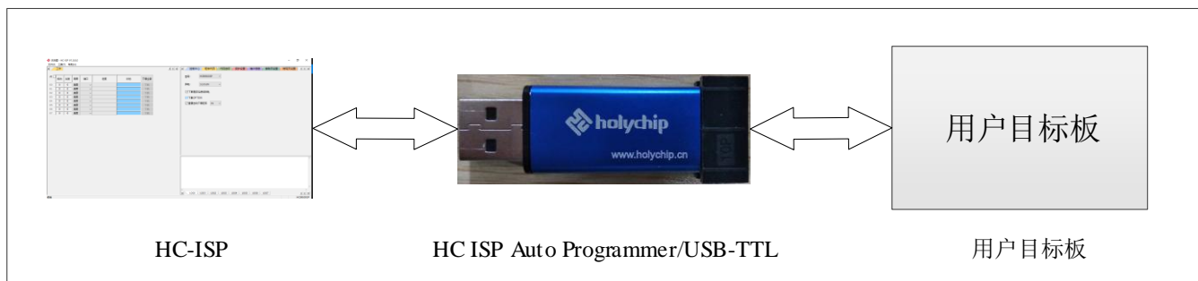
Figure 2-1 硬件连接(HC ISP Auto Programmer)
